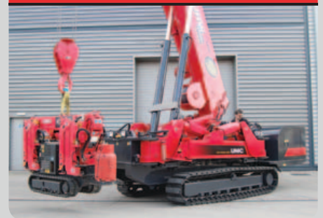
Outriggers stowed to traverse a narrow opening
